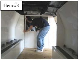
Attach Front Bulkhead to Driver-side Bench/Wall assembly
